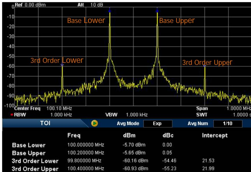
Figure 2-20 TOI Measurement Interface
