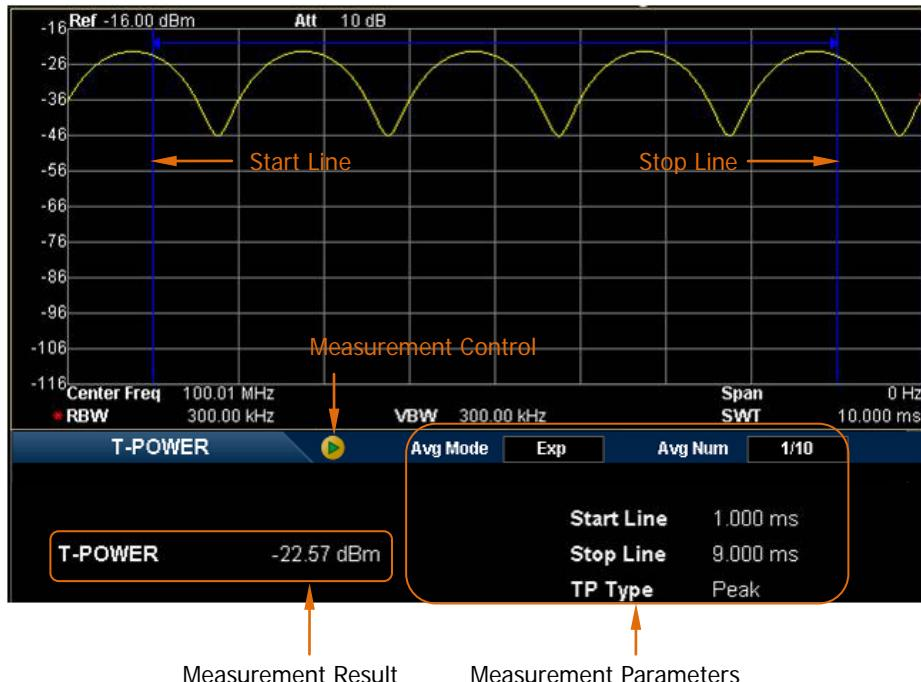
Figure 2-13 T-Power Measurement Interface
