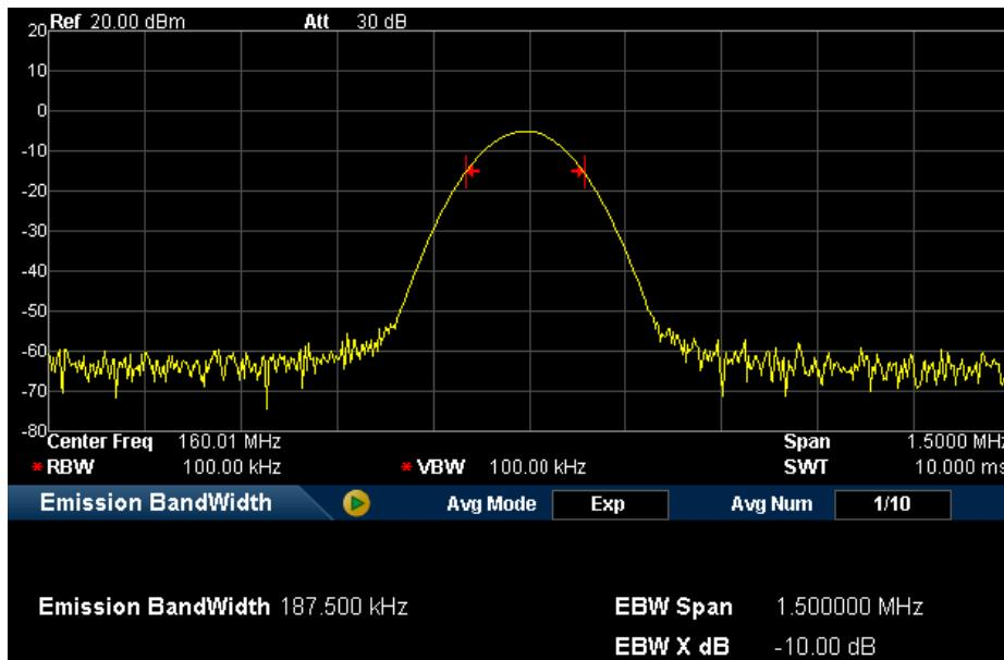
Figure 2-17 EBW Measurement Interface
