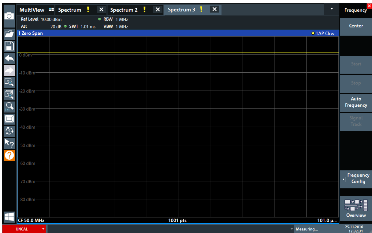
Figure 6-7: Time domain display of the calibration signal
