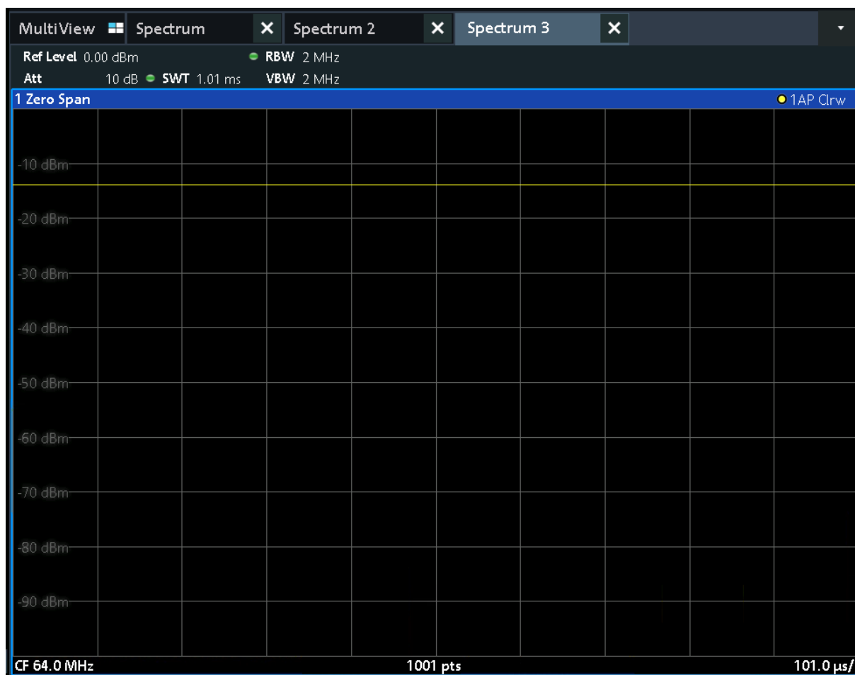
Figure 6-7: Time domain display of the calibration signal
