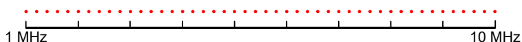
Figure 6-25: Linear x-axis scaling: the distance between the sweep points is equal, e.g. 200 kHz
