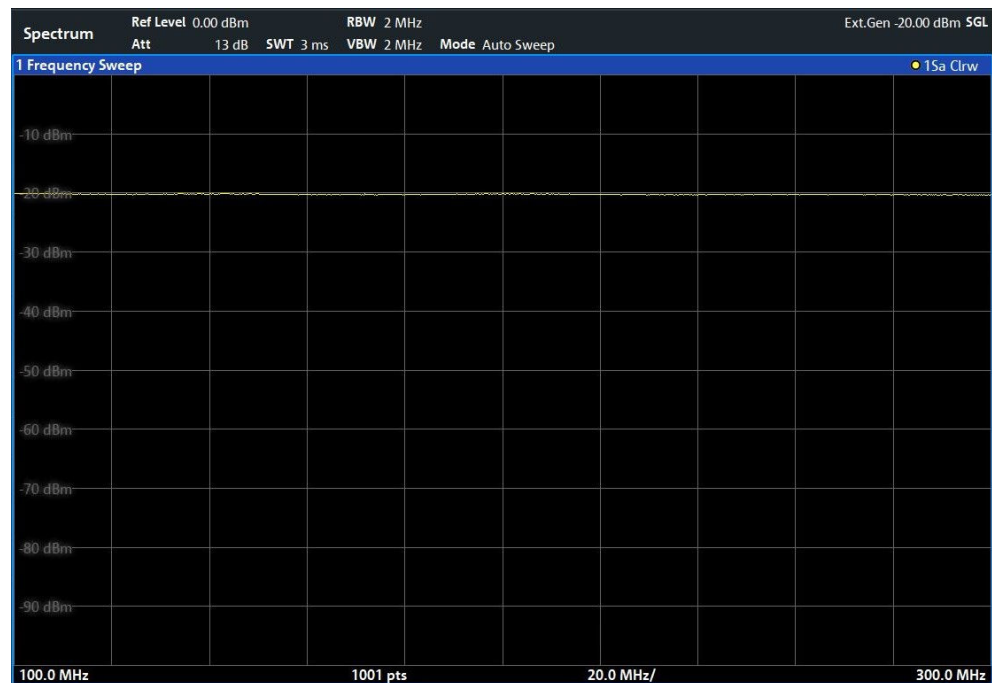
Figure 6-8: Measurement results from generator, analyzer and connecting cables
